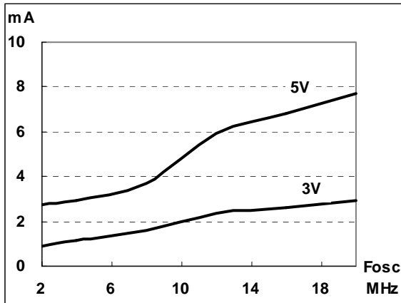
Figure 13-7 Typical Run Mode current ( I_{dd1} ) vs. F_{osc} (Low Power Disable)
